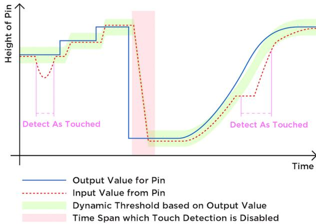
Figure 7. Example Image of Touch Detection Processing.
