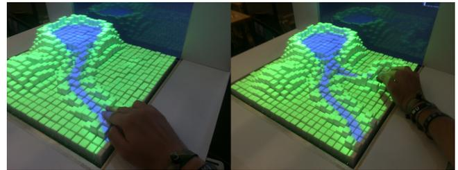
Figure 9. Manipulating and simulating landscapes with flexible, elastic and viscous rendered material properties.
