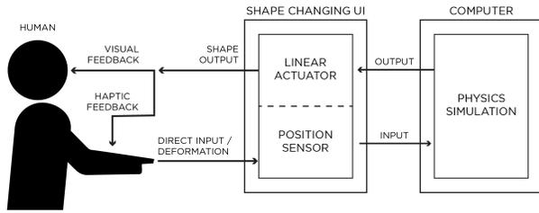
Figure 2. Interaction framework to represent material property using shape changing interfaces.
